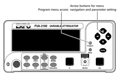
**2.** Press ENTER. The first digit will start flashing. Use the up/down arrows to change the flashing digit and the left/right arrows to activate the next digit.
