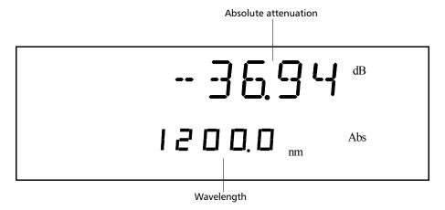
In Offset mode, the offset value is always displayed in the lower portion of the display while the upper portion (large digits) displays the sum of two values.
