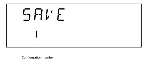
**4.** Press ENTER. The configuration number will start flashing.
