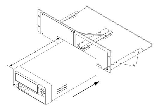
**2.** If a second benchtop is to be installed, remove the cover plate and repeat step 1.
